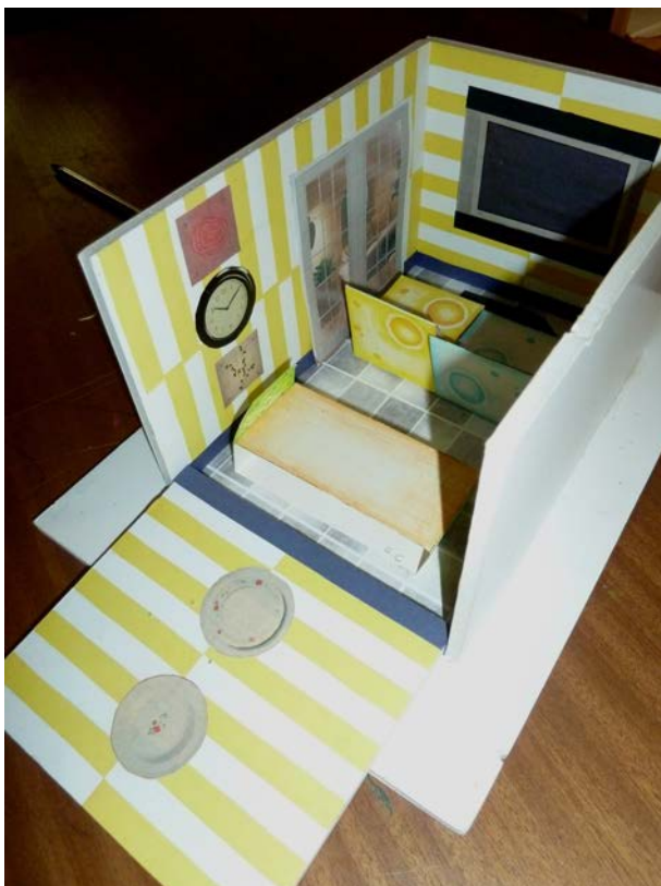
Striped wallpaper made by applying strips of coloured paper to white foamboard walls.
