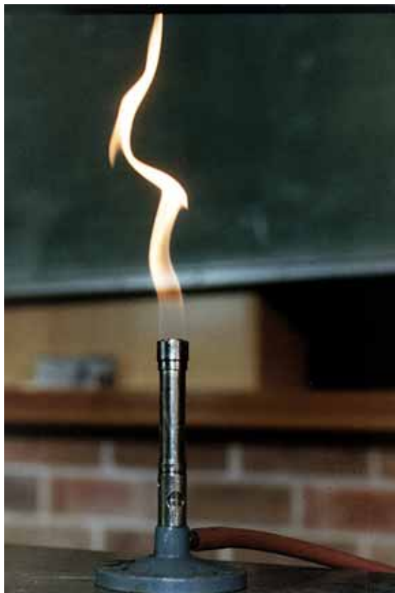
The yellow flame of a Bunsen burner
