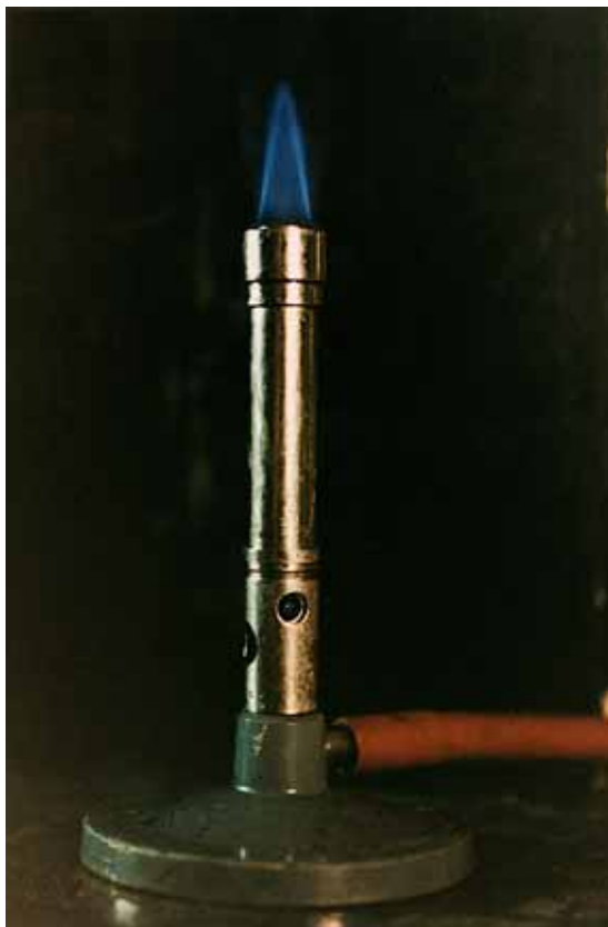
The blue flame of a Bunsen burner
